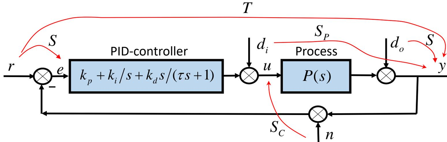
$H(s, k = [k_p, k_i, k_d, \tau]) \triangleq W(s)S_*(s, k)$ ,  $S_* \in \{S, T, S_C, S_P\}$  ..... weighting sensitivity function
