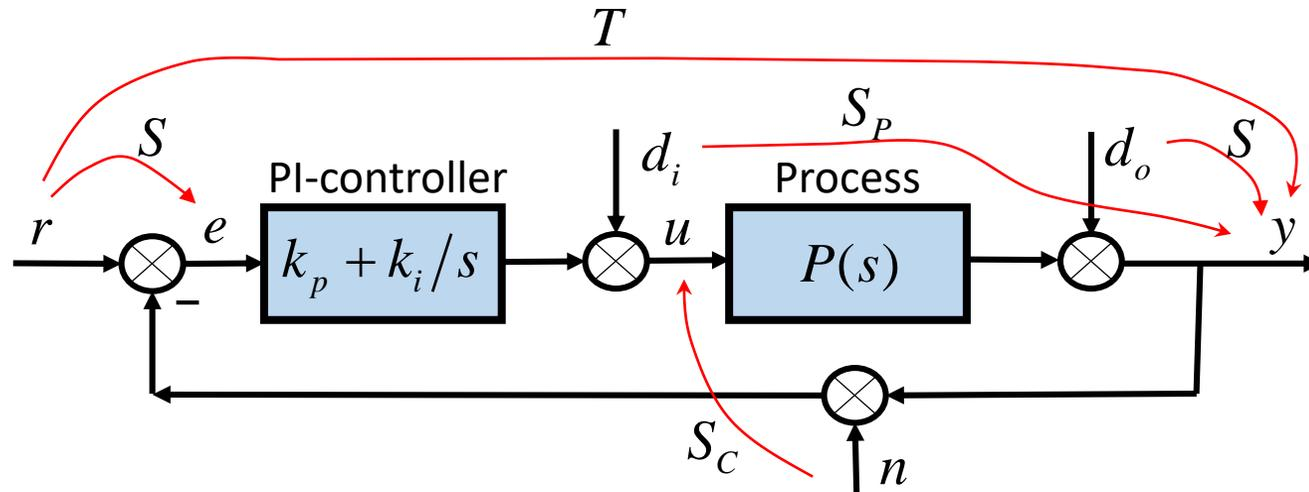
$H(s, k = [k_p, k_i]) \triangleq W(s)S_*(s, k)$ ,  $S_* \in \{S, T, S_C, S_P\}$  ..... weighting sensitivity function
